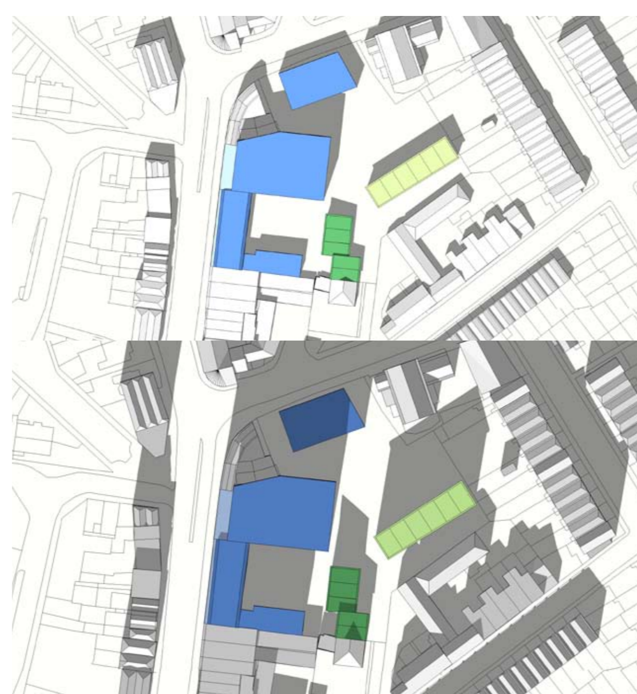
C Above: Shadow plan illustrating typical summer (top) and autumn / spring (bottom) shading conditions anticipated at 12 noon
